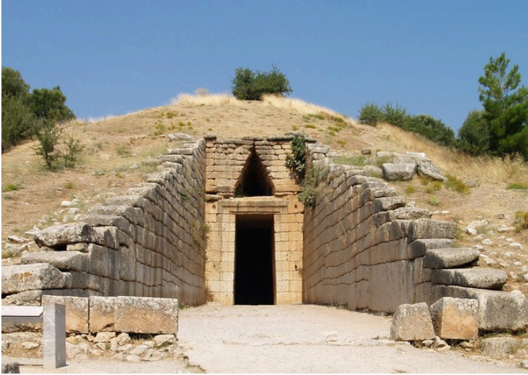
Treasury of Atreus, Mycenae, Greece, circa 1300–1250 BCE.: The Treasury of Atreus and others tombs like it are demonstrations of corbeled vaulting that covers an expansive open space
